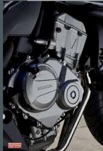
Motor, 4 Zylinder, 78 PS
